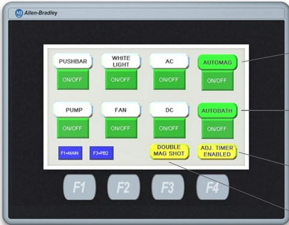
Automatically clamps the part, magnetizes the part, then unclamps the part
